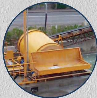
Recycling System for RMC
